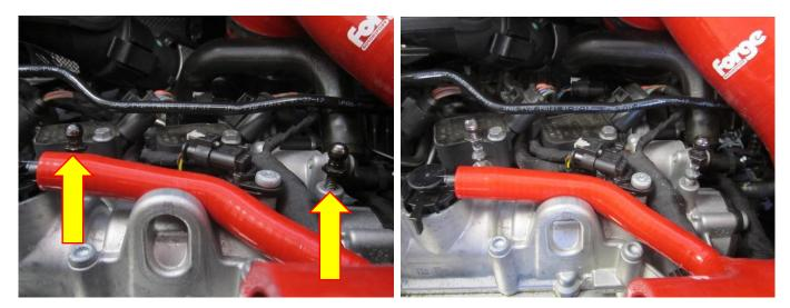
10. Remove the two rubber mounting grommets from the air box, use a flat blade screw driver or trim tool to remove them from the air box. Take your time as they are tightly fitted.
