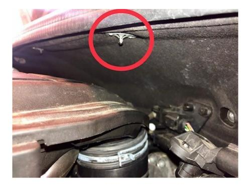
4. Now you will be able to remove the air box from the engine bay, this should just pull out
