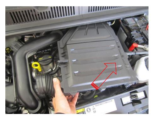
5. With the air box removed from the vehicle, locate the oil breather outlet and remove the rubber hose. The plastic breather outlet needs to be re-positioned. Use a flat blade screw driver or similar to lift the plastic breather upwards so that you can twist it into its new orientation as shown in the bottom picture.
