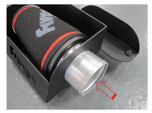
12. Place the Forge hi-flow filter into the heat shield. Fit the 76mm hose joiner to the other end of the Forge cone filter, leaving half of the joiner on show. Use the hose clamp to secure the joiner to the filter.
