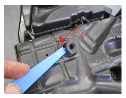
11. Insert the two rubber mounting grommets from the air box and the one supplied with the kit into the Forge heat shield as shown in the picture. You will need to lubricate them to help with fitting.
