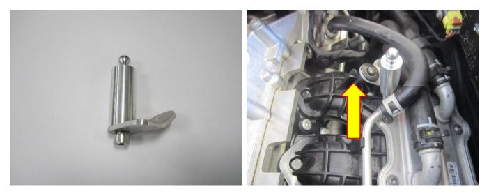
9. Remove the original air box mounting pegs and attach the two steel mounting pegs from the kit on top of the rocker cover
